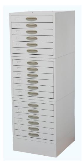
The base is made of SPCC1.2cold-roll steel sheets, the main body and drawers are made of SPCC 0.8 cold-roll steel sheets. This cabinet includes a base and three modules on the top that contains 18 drawers (6 drawers in each module) that accommodate up to 9,000 microscope slides. Numbered labels inside the drawers make filing more convenient.
