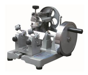
KEDEE KD-202 Rotary Microtome is a simple but practical model. This product consists of a crank driving system and ratchet wheel feeding mechanism, and can provide even and continuous sectioning.
