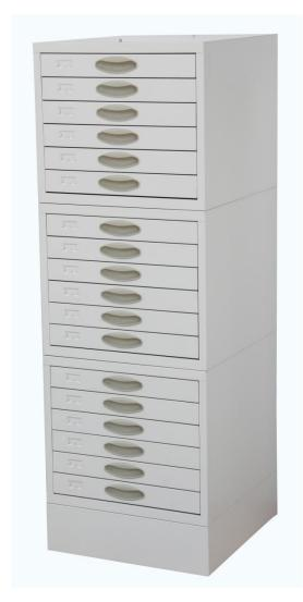
The base is made of SPCC1.2cold-roll steel sheets, the main body and drawers are made of SPCC 0.8 cold-roll steel sheets. This cabinet includes a base and three modules on the top that contain 18 drawers (6 drawers in each module) that accommodate up to 11,000 tissue blocks. Movable dividing boards inside the drawers make filing more flexible.
