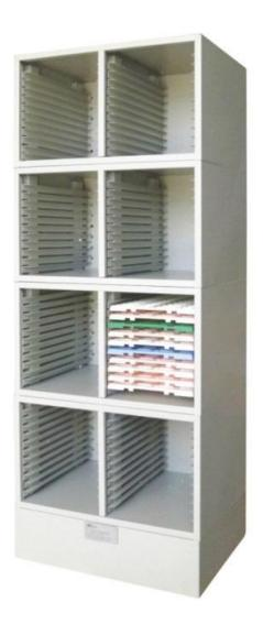
The base is made of SPCC1.2cold-roll steel sheets, the main body and drawers are made of SPCC 0.8 cold-roll steel sheets. This cabinet includes a base and four stacked modules, each module can accommodate up to 96microscope slide-drying boards (24 in each section). The numbered labels in each section make filing more convenient.
